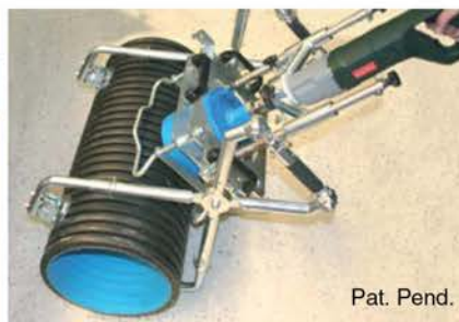
Anboring dy ≤ Ø 658 mm beton/plast
