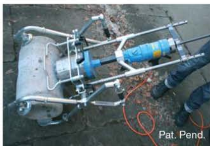
Anboring dy ≤ Ø 658 mm beton/plast
